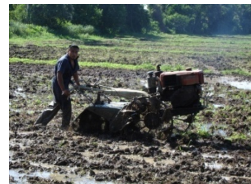
Fig. 6: Land prep. with rotortillers
